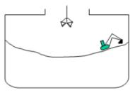
If the load has a fluid structure, the dotted line in the figure on the right side decreases as the line is discharged. The duration of evacuation and cleaning is shortening.
