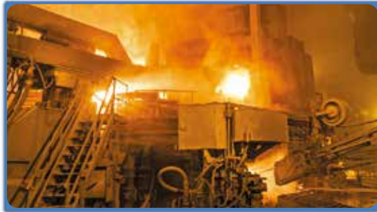
MELTING OF STEEL SCRAP IN EAF
